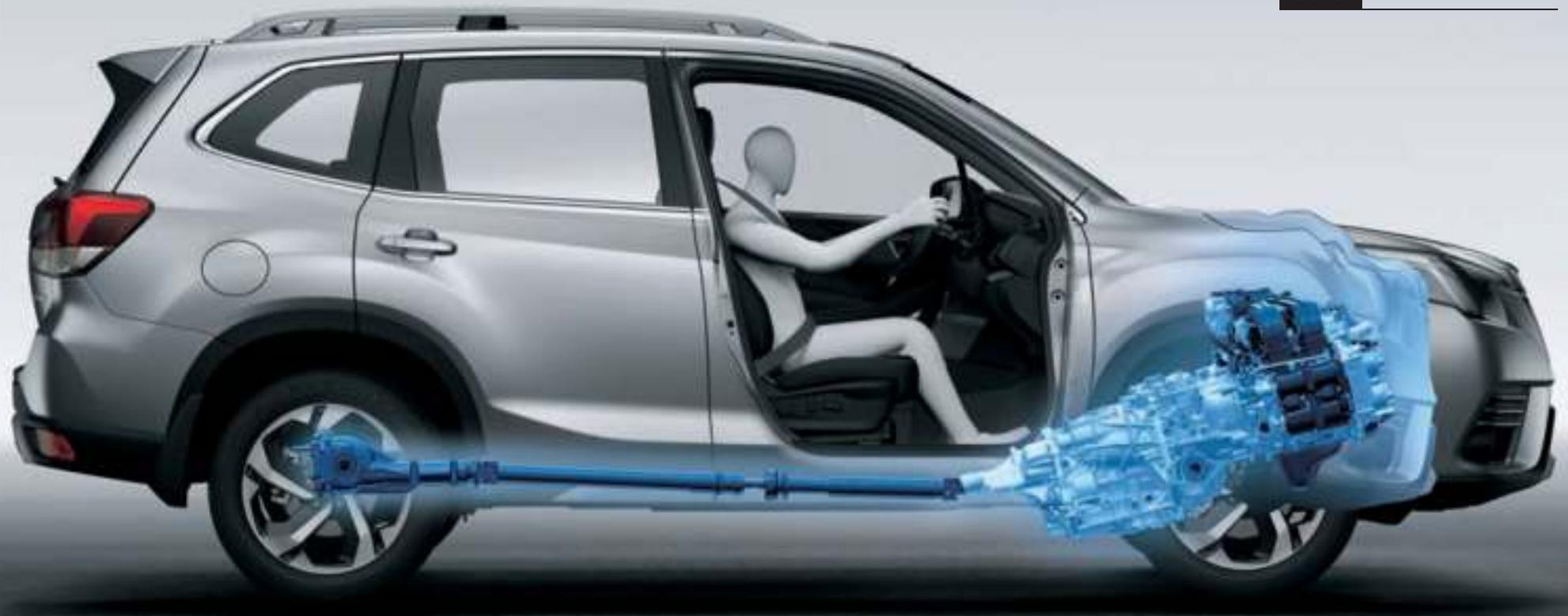
Designated crumple zones direct impact energy away from the passenger cell, while the Boxer engine is designed to slide below the cabin in a severe frontal collision.
