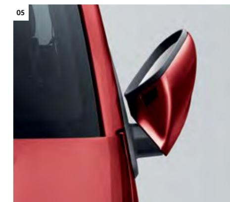
**05 Electrically adjustable, heated, folding door mirrors.** Automatically folded to the vehicle when the vehicle is locked by means of remote control. | CP | CE | H |
