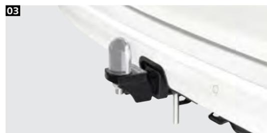
**03 Tow bar kit.** The Volkswagen Multivan towbar is designed for perfect integration with your vehicle chassis and tested to meet the stringent Australian and Volkswagen engineering standards. The genuine electrical installation kit provides the electrical supply, and ensures that the trailer can be operated safely. Full integration into the vehicle's CAN-bus network is provided for all components, including support for the vehicle-trailer stabilisation system.
